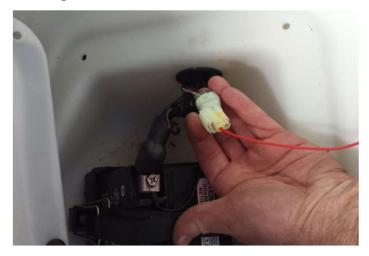
Use zip ties to attach the black plastic wire loom away from hot engine parts. Trim the black plastic so that only the red wire passes through the edges of the panels. Replace the panels by pressing the black clips in place
